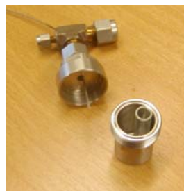
Reusable metal cell with glass insert and thermocouple liner
