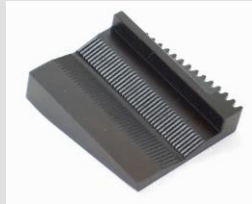
J243-BV30: Special jaws for round samples 30mm Ø
