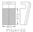
J122SK Coarse serrated face for samples 1 (0.4") to 12 mm (0.48") thick..
