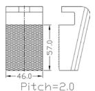
J122BP diamond or pyramid serrated face for samples 1 (0.4") to 12 mm (0.48") thick
